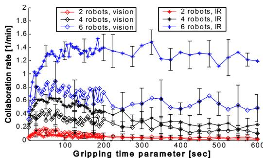
Figure 8: For a scan interval of 30 cm and scan angle of  $360^\circ$ , the advantage of the larger field of view of the IR team is apparent.
