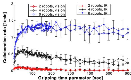
Figure 7: For a scan interval of 70 cm and scan angle of  $360^\circ$ , the performances of both teams are equivalent.
