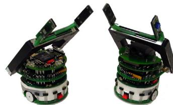
Figure 2: Khepera robots equipped with gripper and IrDA modules (left), and gripper and camera modules (right)
