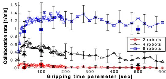
**Figure 9:** Real robot experiment results and the Webots data for the same parameters. Solid color markers represent the results for real robot experiments.
