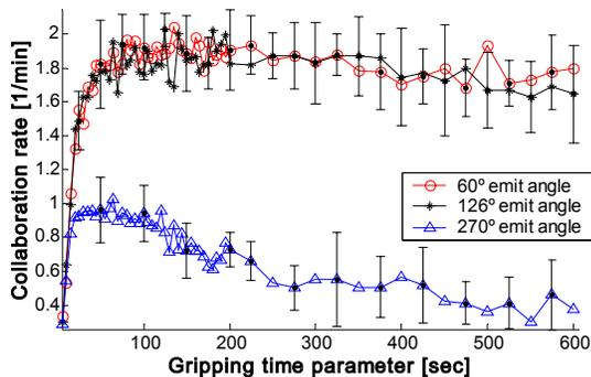
Figure 3: Performance of a group of 6 robots for different IR emission angles.
