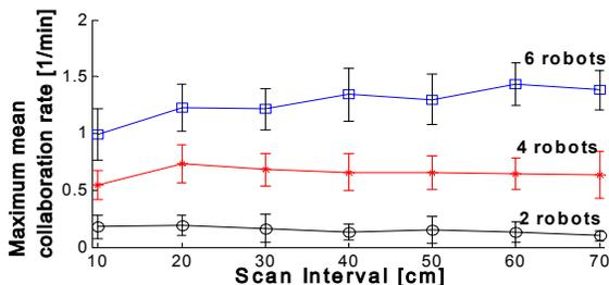
Figure 5: Maximal performance for each scan interval, with scan speed of 1 revolution per 21 seconds.
