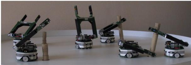
Figure 1: Physical set-up for the stick-pulling experiment
